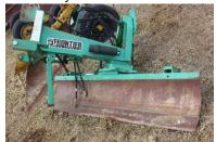
\* Frontier 3pt. back blade. Both tilt & front/back hyd. SN RB2307
